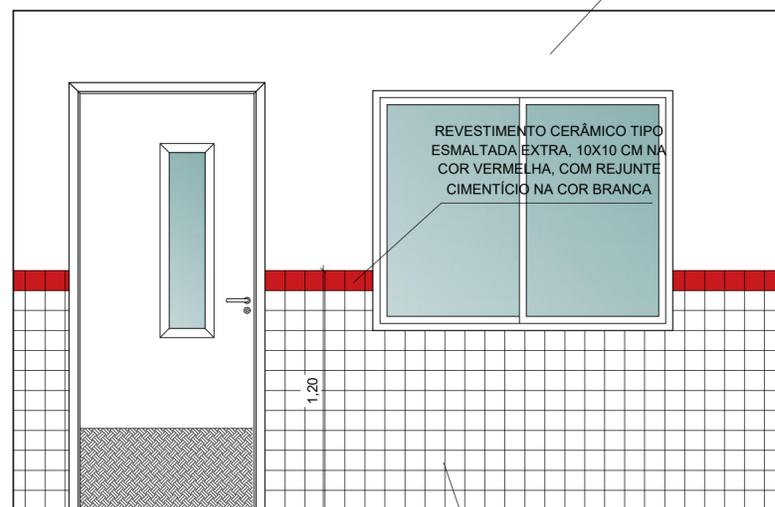
REVESTIMENTO CERÂMICO TIPO ESMALTADA EXTRA, 10X10 CM NA COR BRANCA, COM REJUNTE NA COR BRANCA
